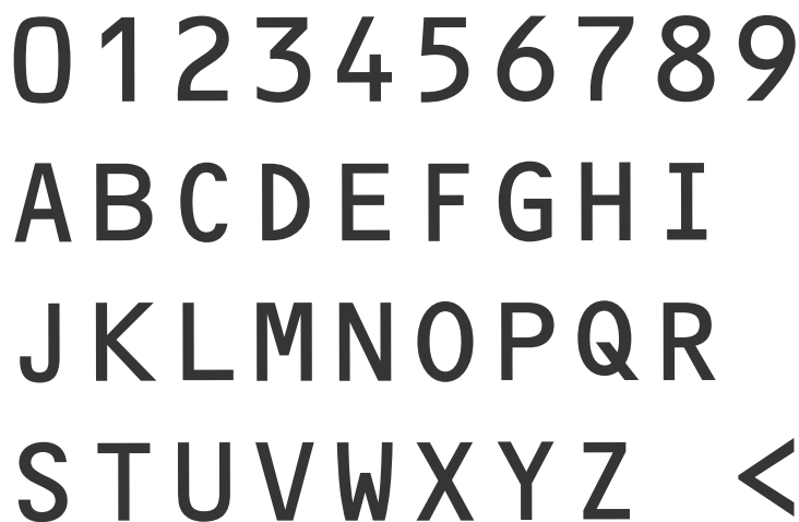
Figure 4. Subset of OCR-B Characters from [ISO 1073-2] for use in machine readable travel documents
